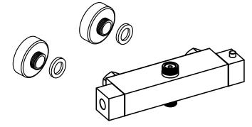
**Step 2** Install the main body and rubber pad.
