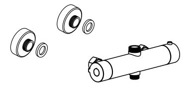
**Step 2** Install the main body and rubber pad.
